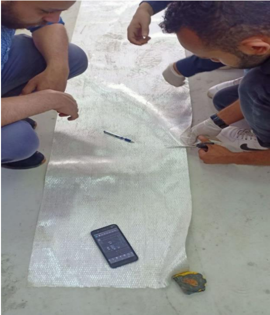
Figure (3-29-b1): Cutting of GFRP sheet to the required dimensions
