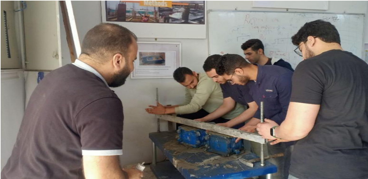
Figure (3-4): Casting and compaction of concrete mix
