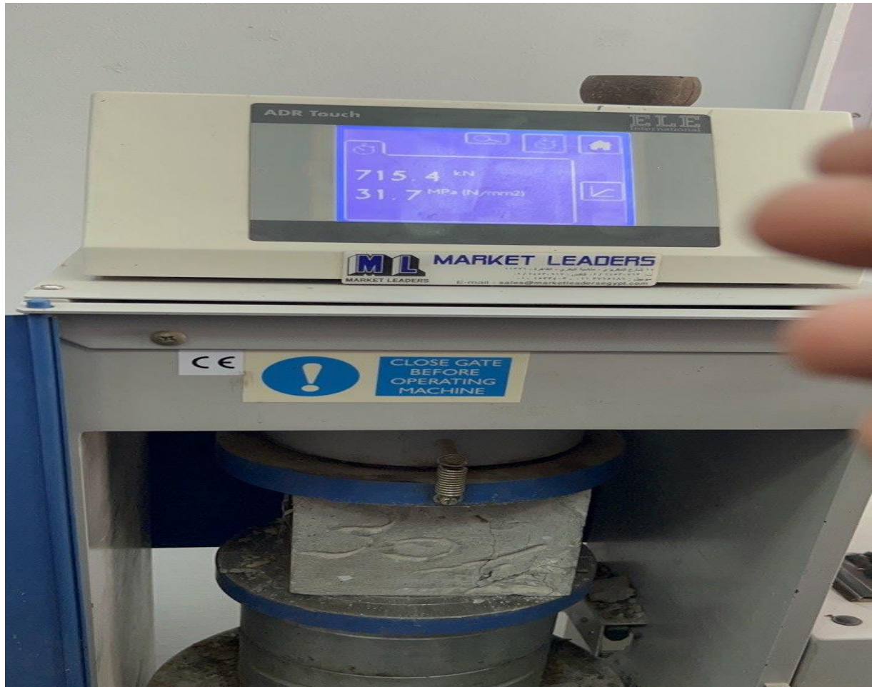
Figure (3-7): Compressive load test
