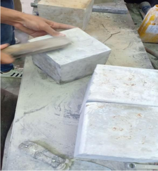
Figure (3-29-a): Smoothing the concrete surface for the specimen
