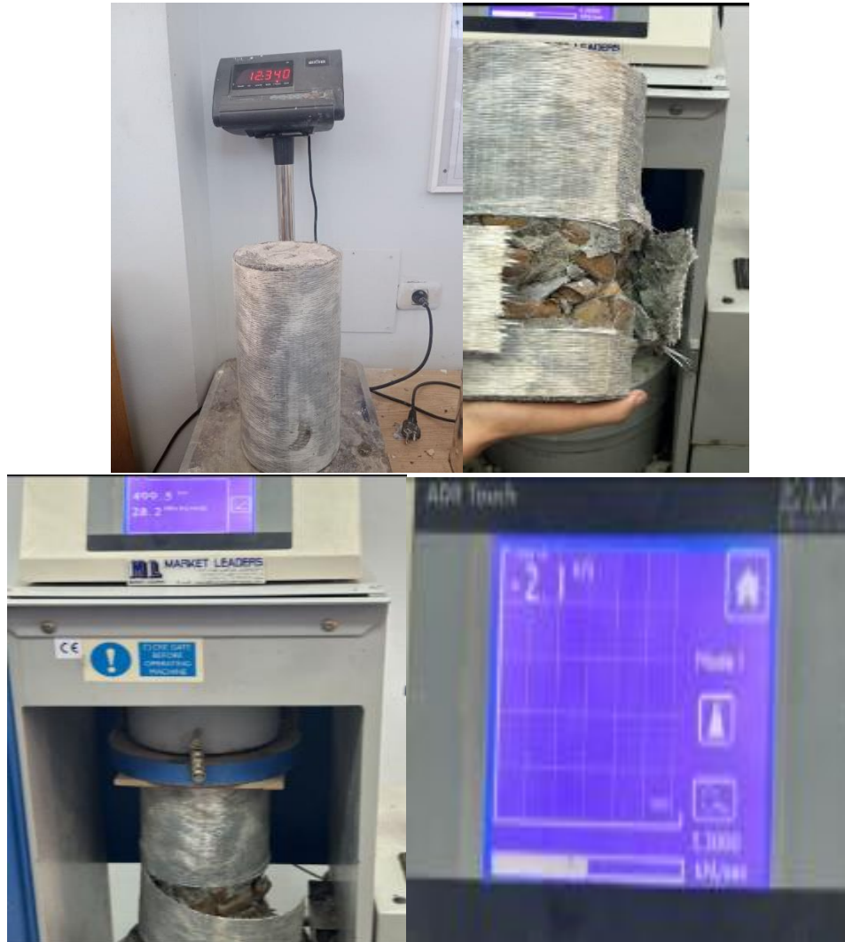
Figure 4.5 Failure shape of S6
