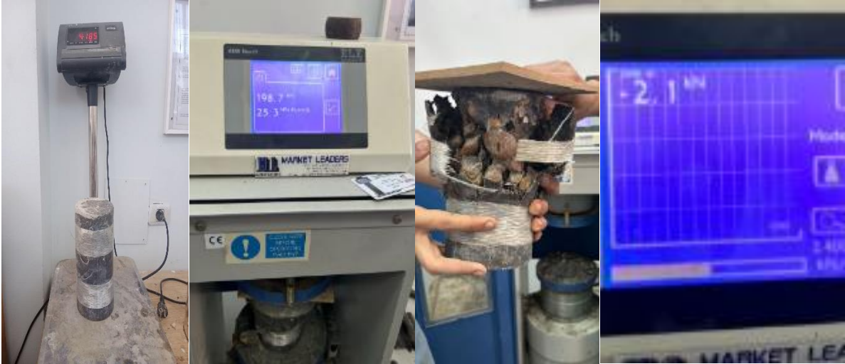
Figure 4.14 Failure shape of S13
