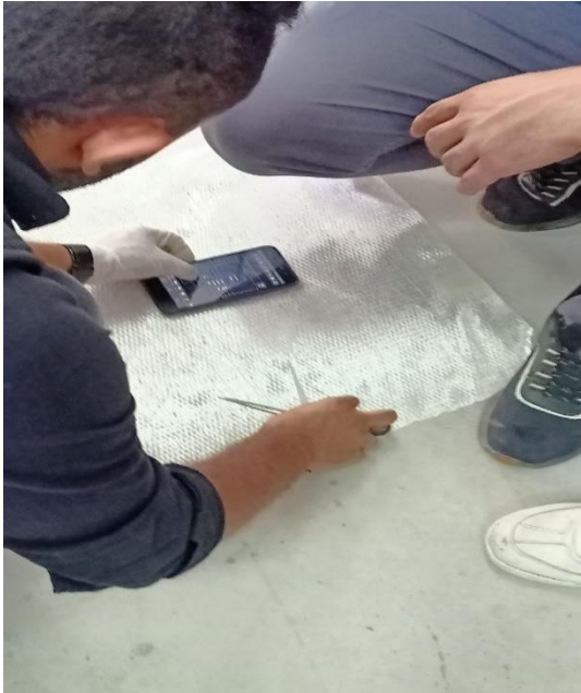
Figure (3-29-b1): Cutting of GFRP sheet to the required dimensions
