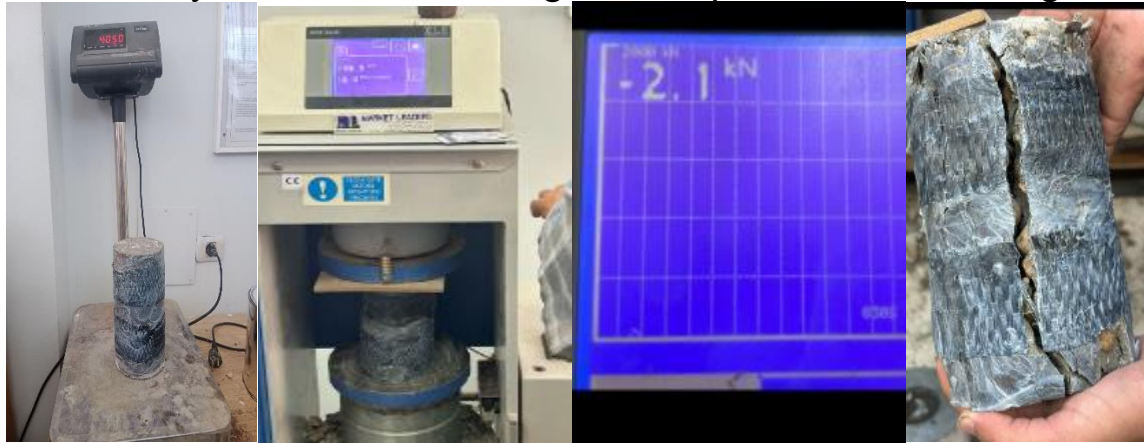
Figure 4.19 Failure shape of S18
