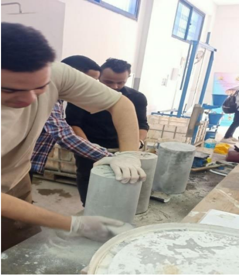
Figure (3-29-a): Smoothing the concrete surface for the specimen
