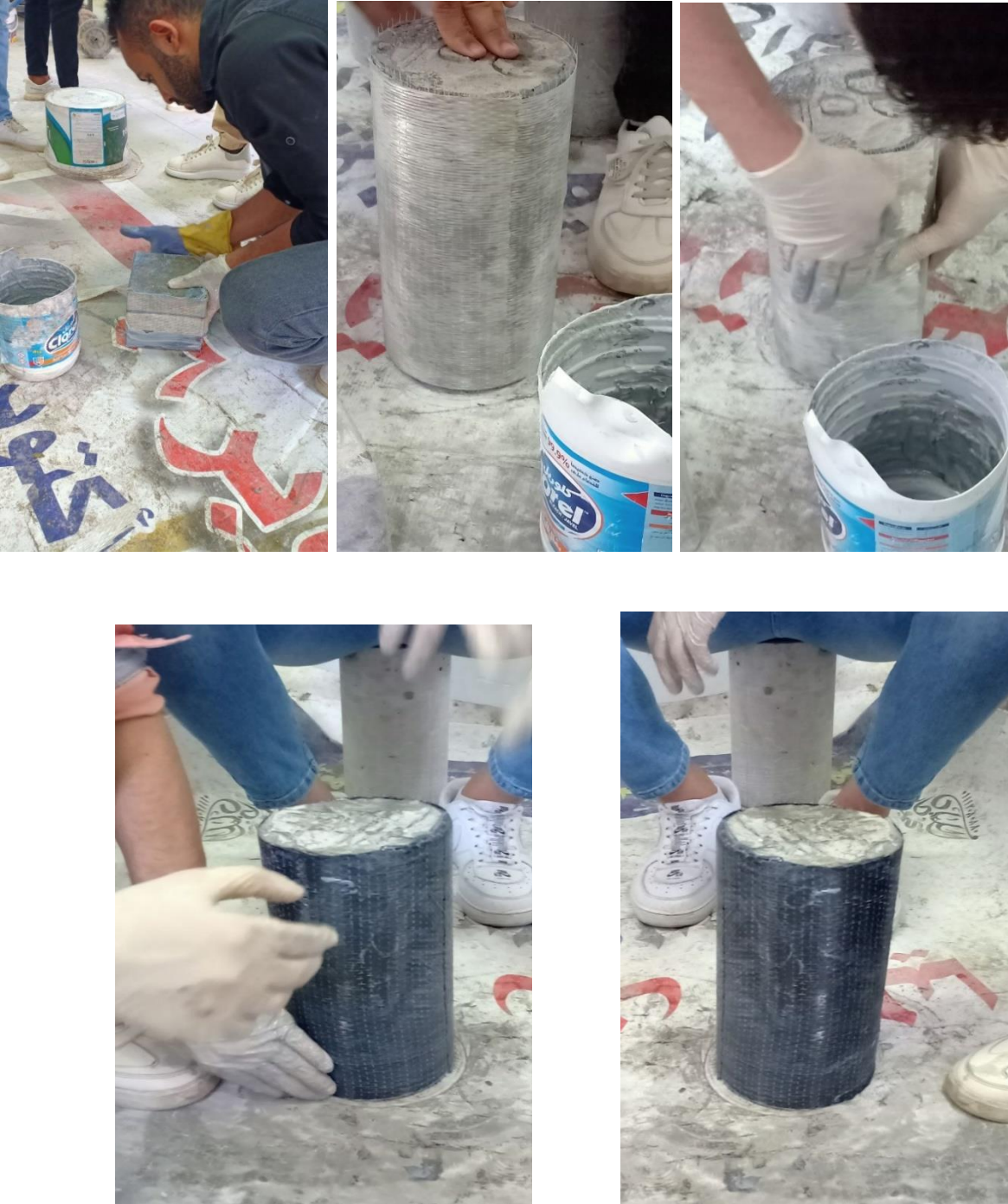
Figure (3-29-e): Applying the second layer of epoxy
