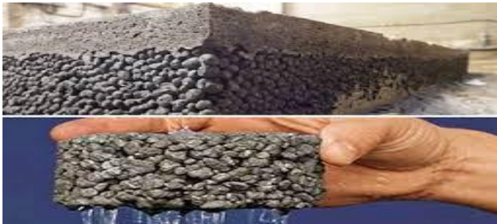
Figure 3-3 No Fines Concrete
