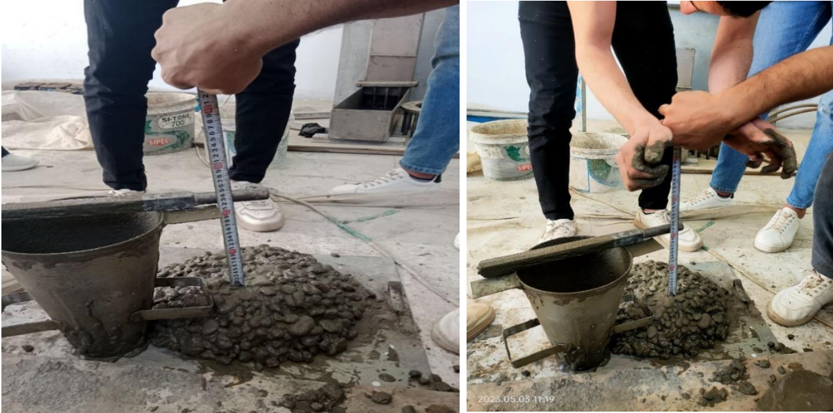
Figure (3-6): Testing of fresh concrete(The slump test)
