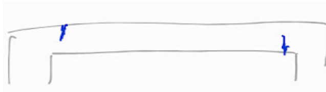
(Subsidence cracks of one of the pillars in the beams)
