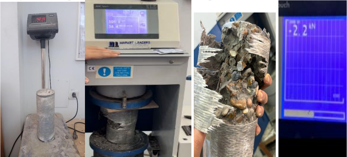
Figure 4.16 Failure shape of S15
