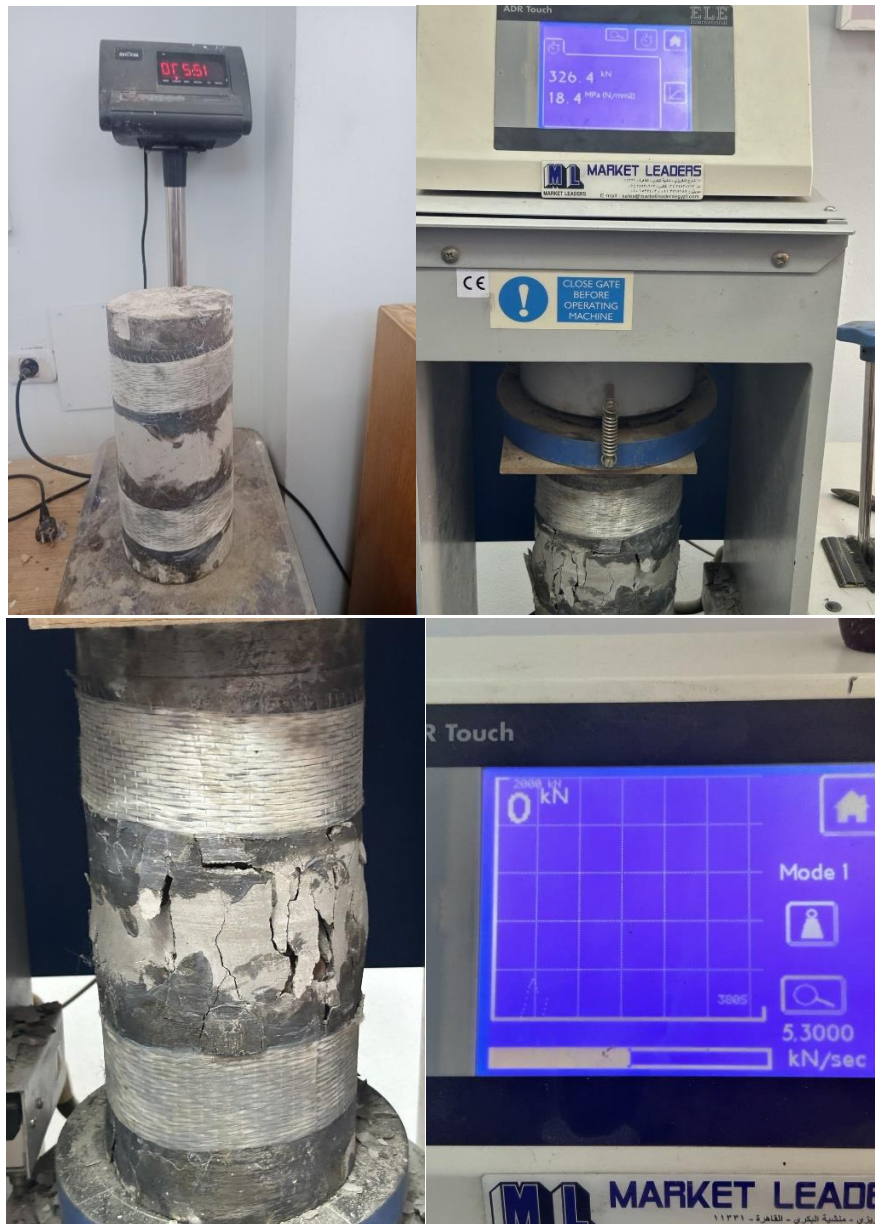
Figure 4.3 Failure shape of S4
