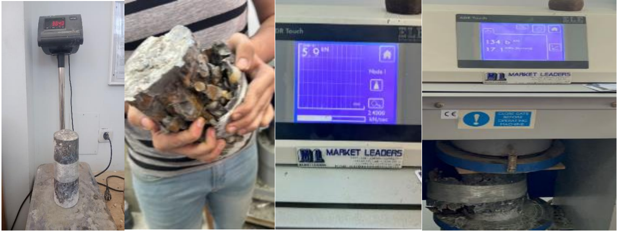
Figure 4.17 Failure shape of S16
