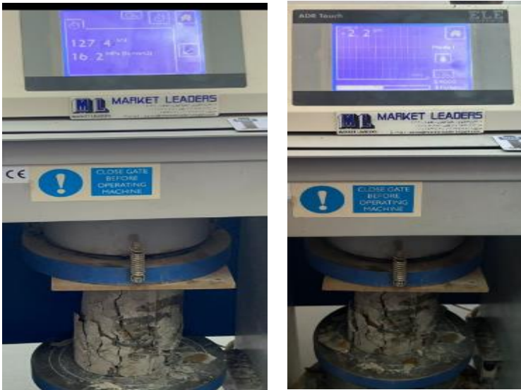
Figure 4.13 Failure shape of S3
